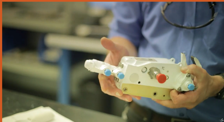
Héroux-Devtek’s F-35 landing gear door uplock mechanism (Screengrab/Lockheed Martin). 24
