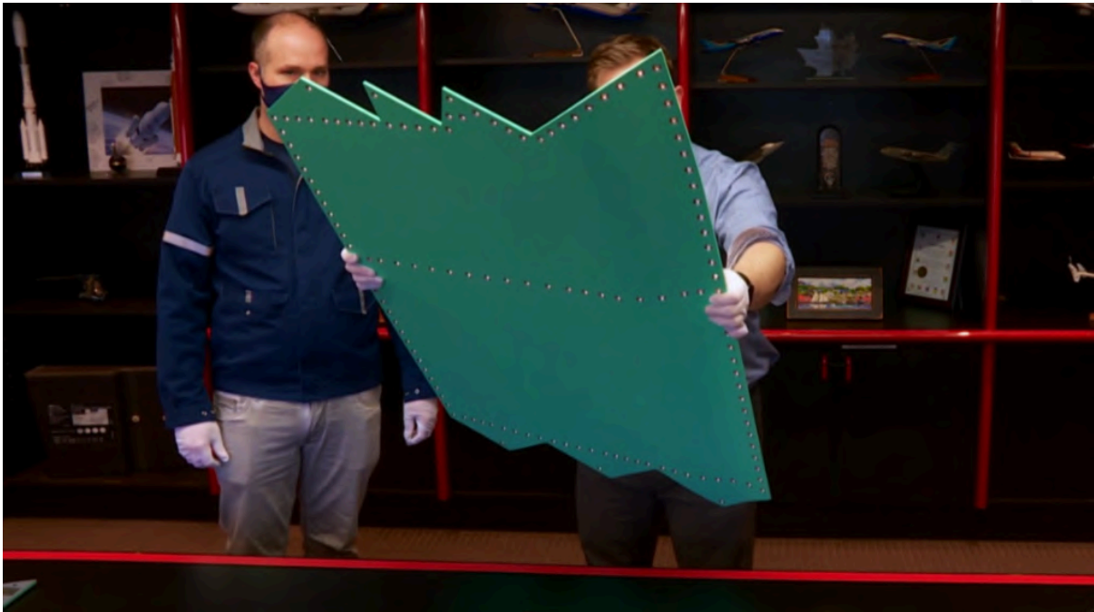
[Fig. N: A Stelia composite panel for the F-35 (Screengrab/CBC). 34 ]
