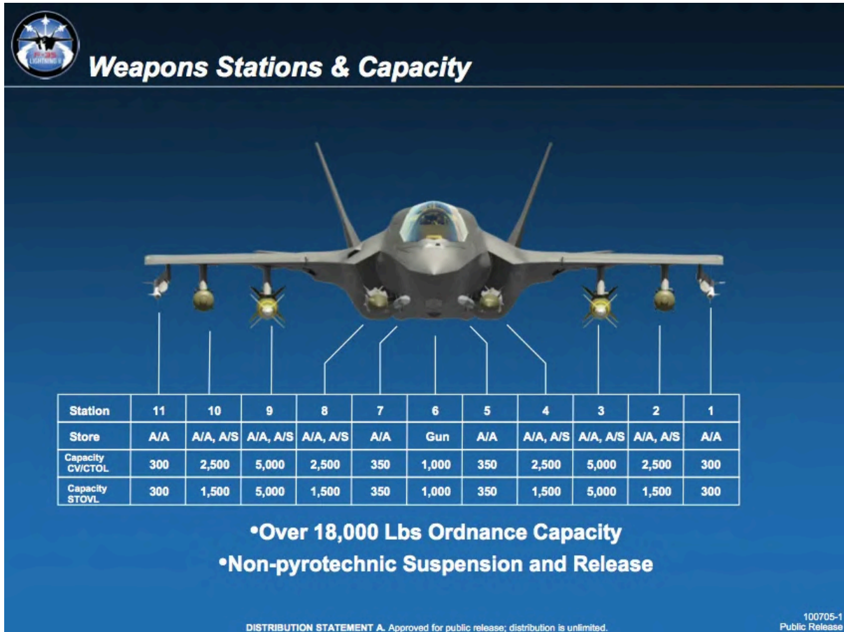
[Fig. N.: Diagram of F-35 payload capacity (F-35 Joint Program Office via The War Zone ). 88 ]
