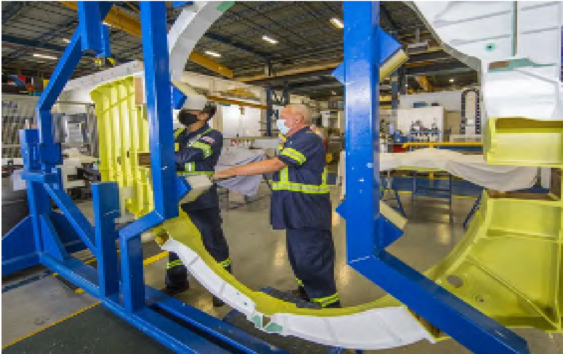
[Fig. N.: F-35 bulkhead being worked on at Asco factory (Francis Georgian /PNG). 6 ]
